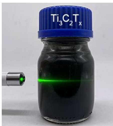
Fig. S3 The Tyndall phenomenon of the as-obtained \text{Ti}_3\text{C}_2\text{T}_x MXene suspension.
