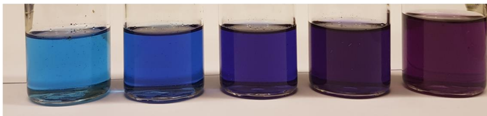
Figure S24. The effect of relative permittivity on Brooker's merocyanine dye solution in CH 2 Cl 2 in a control experiment. Upon addition of NBu 4 PF 6 the relative permittivity is changed from 8.93 to 24.2, 20 resulting in color change from light-blue to violet. Worth noting is that solution of the dye in acetone with \epsilon=20.7 is also violet.
