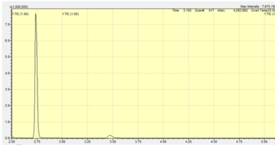
Fig. S28: Representative GC-MS-trace of product gas stream obtained with MEAs featuring the Pn-type cathodes. The Signals correspond to H 2 and O 2 , respectively.
