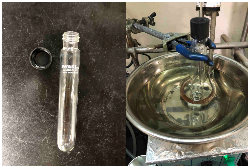
Figure S2. Photos of a 20 mL screw cap test tube used in this study: reaction set up (left); reaction progress (right).
