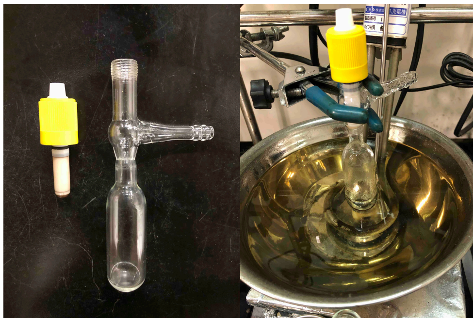
Figure S1. Photos of a schlenk flask used in this study: reaction set up (left); reaction progress (right).
