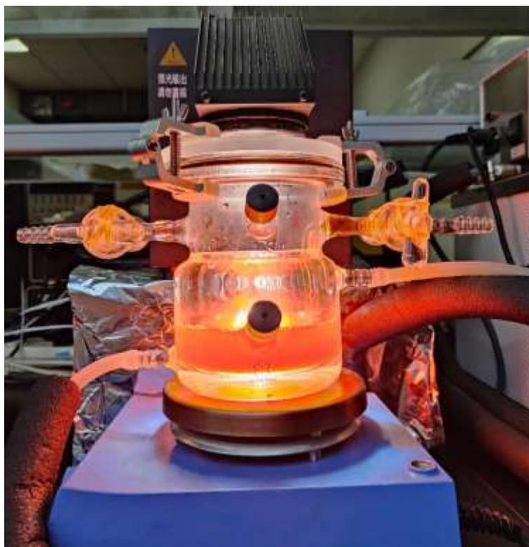
Figure S46. The picture of photocatalytic reactor.
