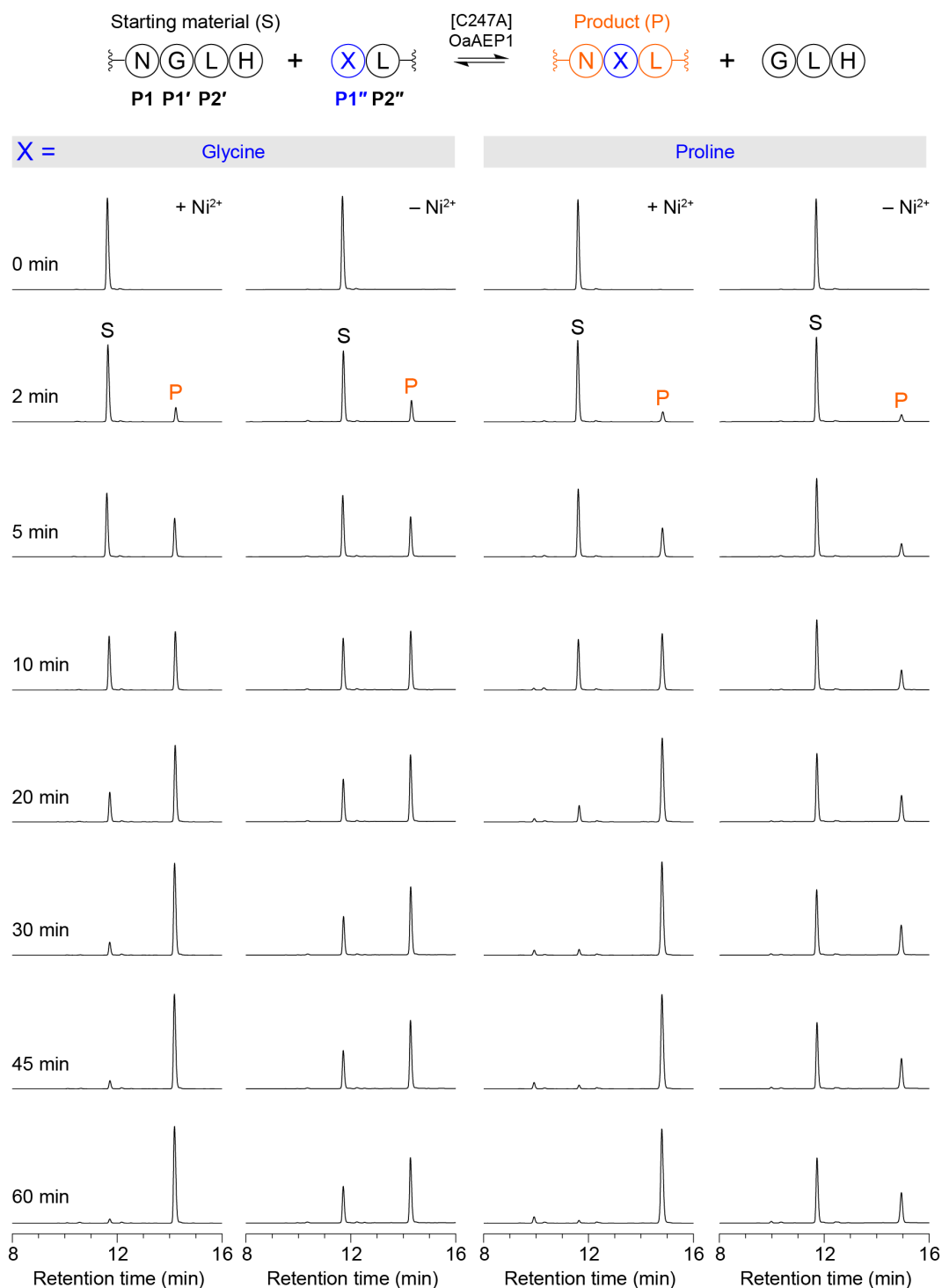
Figure S4. Time course for ligation of GLRL or PLRL to a model NGLH substrate. Reactions were run as described in Figure S1 in the presence (+) or absence (-) of 300 \mu M NiCl 2 (as indicated). At the indicated time points (left panels), reactions were quenched by addition of TFA (1%) prior to analysis. Shown are representative analytical reverse-phase HPLC traces (A280 nm) from three experiments. Peaks for starting material (S, black) and product (P, orange) are indicated.
