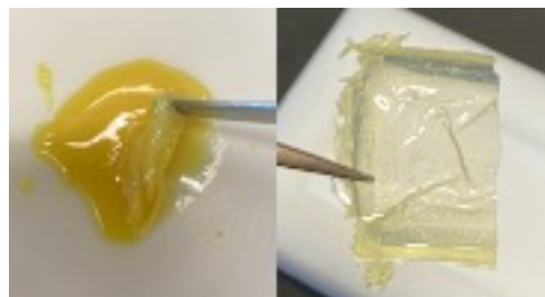
Figure S8. Photographs of MMMs using varied wt% of UiO-66-NH 2-170 MOF particles after 3 h polymerization. Left: Incomplete polymerization resulting in a viscous mass of 30 wt% UiO-66-NH 2-170 /P1. Right: Free-standing membrane of 0.7 wt% UiO-66-NH 2-170 /P1 MMM.
