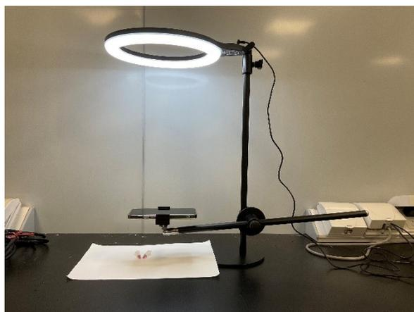
**Fig. S1** Setup image for the colorimetric analysis
