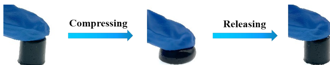
Figure S1 Deformations of the the PAA/Starch/MXene organohydrogel with compressing and releasing states.
