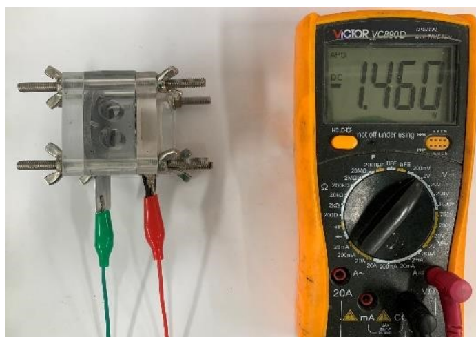
Figure S15. Image of the ZAB with a measure open-circuit voltage of 1.46 V.
