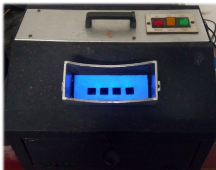
Figure S9 Digital image of the experimental setup of UV irradiation on the perovskite layer.
