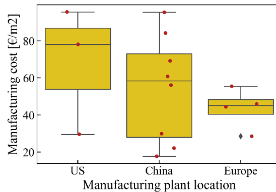
Figure S1. Perovskite module cost as a function of the manufacturing plant location.
