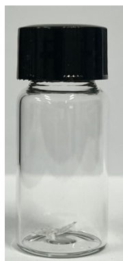
Supplementary Fig S6: white crystals from evaporation of washing solution.
