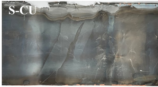
Supplementary Fig S2: comparison of graphite copper foil stripped by heat treatment
