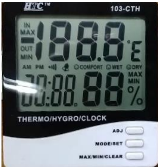
Fig. S9. Powering up a digital hygrometer by using the stored charge of a 10 \mu F capacitor (using the rectified output of BTS15W-based HNG).
