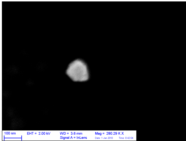
Figure S3: SEM image of a PNIPAM-PEGMA particle in the collapsed, dehydrated state.
