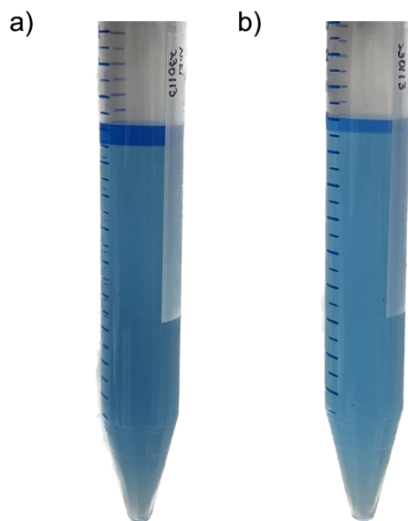
Figure S4. Phase separated solutions consisting of a) 5 ml of DEX 30 w/v% and 5 ml mixture of DEX 5 w/v%, PEG 1 and Alexa Fluor 1 \mu\text{l ml}^{-1} and b) 5 ml of DEX 20 w/v% and 5 ml mixture of DEX 5 w/v%, PEG 1 and Alexa Fluor 1 \mu\text{l ml}^{-1} .
