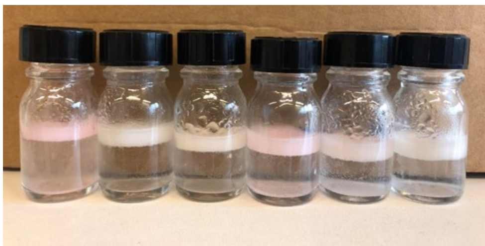
Figure S3. Pickering emulsions made with 25 mg of particles per \text{cm}^3 of oil. From left to right N-, A-, C-, A/N-, N/C- and A/C-emulsions. The picture was taken 4 months after the preparation of emulsions. No release of free oil was observed on top of the emulsions.
