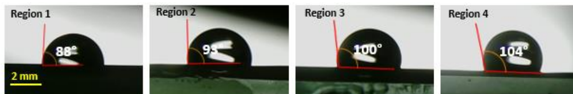
Figure S6. Contact angle measurements of wettability gradients formed on Ecoflex 00-30 Platinum Cure Silicone Rubber Compound.
