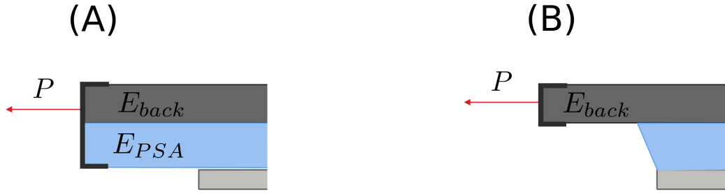
Fig. S8 Scheme of the lap shear experiment illustrating the free region of PSA Figure (A). If the free region of PSA is neglected then Figure (B) is an accurate representation.
