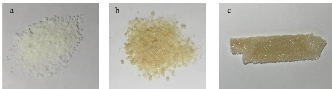
Figure S2 Optical photograph of (a) ZIF-62 crystal; (b) Powder ZIF-62 glass; (c) Bulk ZIF-62 glass.
