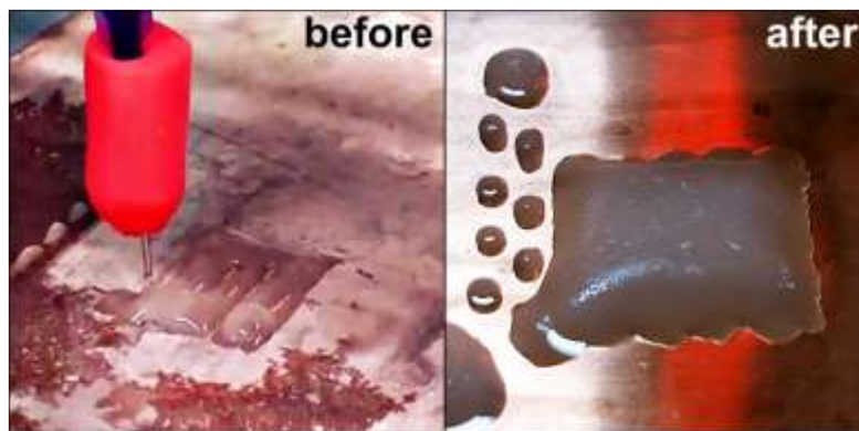
38 Figure SI.2. Photographs demonstrating the preliminary POC printability of a 0.5% FucoPol solution. The left and right panels 39 correspond, respectively, to a printed FucoPol structure before and after complete structural freezing of the liquid fraction.
