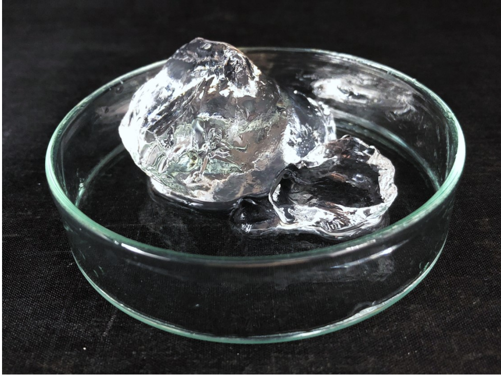
Fig. S4. Photograph of the collapsed chitin hydrogel (DA = 78.8%).
