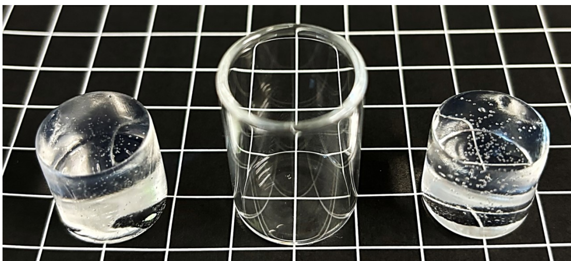
Fig. S1. Photograph of chitin alcogel with sufficient \text{Ac}_2\text{O} (left, DA = 99.4%), cylindrical mould (centre), chitin alcogel with insufficient \text{Ac}_2\text{O} (right, DA = 81.7%). The grid square represents 1 cm.
