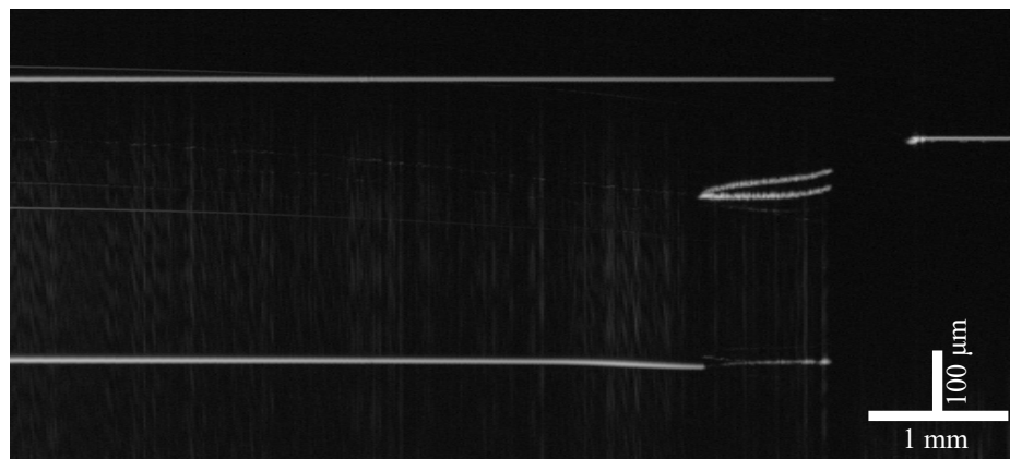
Fig. S4 A cross-sectional OCT image of drying SM-30 suspension ( d = 10 nm) inside a drying cell where cell height H = 300 \mu\text{m} . The initial volume fraction of the suspension \phi is 0.20 and the image was captured 40 min after the suspension is injected into the cell. An internal crack is visible on the upper-right of the image, appearing as two bright lines in proximity. The reflection from the suspension-glass interface below the crack is blurred and suppressed in intensity.
