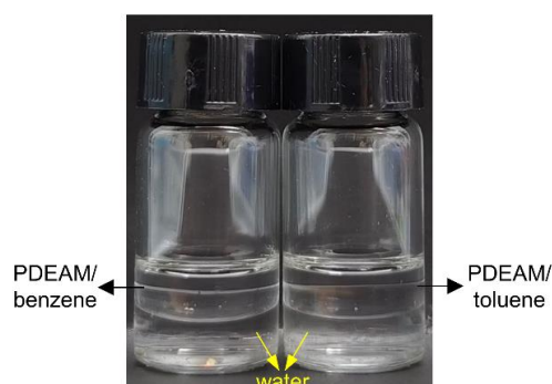
Fig. S6 Optical photograph of benzene and toluene solutions dissolved with PDEAM ( 2 \text{ mg mL}^{-1} , 1 \text{ mL} ) contacted with bottom water ( 1 \text{ mL} ). Photograph was taken after 1 h.
