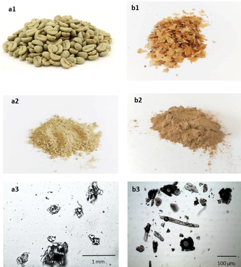
Fig. S1 - Processed biomasses. a1) image of green coffee beans; a2) image of blended green coffee beans; a3) optical microscope images of blended green coffee beans; b1) image of silverskin; b2) image of micronized silverskin; b3) optical microscope images of micronized silverskin.
