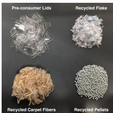
Fig. S1 Pre-consumer lids were the main PET plastic used in these studies unless otherwise stated and are EcoProducts cold drink lids containing 25% recycled content. Recycled PET materials were provided by Verdeco. Recycled pellets are from food grade PET plastics. Plastic bottle pieces were cut up from an Arrowhead water bottle.
