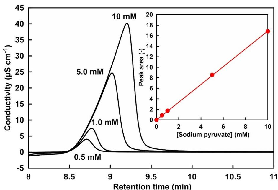
**Figure S1.** Chromatogram of sodium pyruvate (0 - 10 mM) in 50 mM-HEPES buffer (pH 7.0). Inset: Relationship between the sodium pyruvate concentration and the detection peak area.
