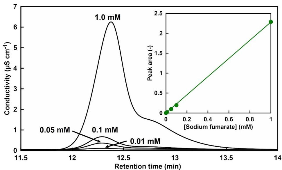
**Figure S3.** Chromatogram of sodium fumarate (0 – 1.0 mM) in 50 mM-HEPES buffer (pH 7.0). Inset: Relationship between the fumarate concentration and the detection peak area.
