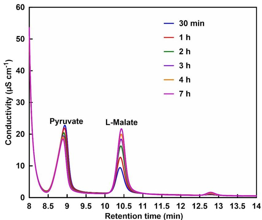
**Figure S4.** A chart of an ion chromatogram for pyruvate or L-malate concentration in the solution of sodium pyruvate (5.0 mM), magnesium chloride (5.0 mM), NADH (5.0 mM) and MDH (0.7 U, *ca.* 1.6  $\mu$ M) in 5.0 mL of 500 mM HEPES-NaOH buffer (pH 7.8). The gas phase: CO<sub>2</sub>.
