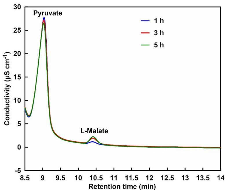
**Figure S6.** A chart of an ion chromatogram for pyruvate or L-malate concentration in the solution of sodium pyruvate (5.0 mM), magnesium chloride (5.0 mM), TEOA (0.2 M), ZnTPPS (10 μM), [Cp\*Rh(bpy)(H<sub>2</sub>O)]<sup>2+</sup> (10 μM), NAD<sup>+</sup> (0.5 mM) and MDH (0.7 U, *ca.* 1.6 μM) in 5 mL of 500 mM HEPES-NaOH buffer (pH 7.8) with irradiation. The gas phase was filled with CO<sub>2</sub> gas.
