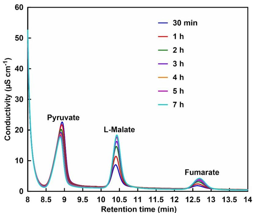
**Figure S5.** A chart of an ion chromatogram for pyruvate, L-malate or fumarate concentration in the solution of sodium pyruvate (5.0 mM), magnesium chloride (5.0 mM), NADH (5.0 mM), MDH (0.7 U, *ca.* 1.6 μM) and FUM (0.5 U; 1.3 nM) in 5.0 mL of 500 mM HEPES-NaOH buffer (pH 7.8). The gas phase: CO<sub>2</sub>.
