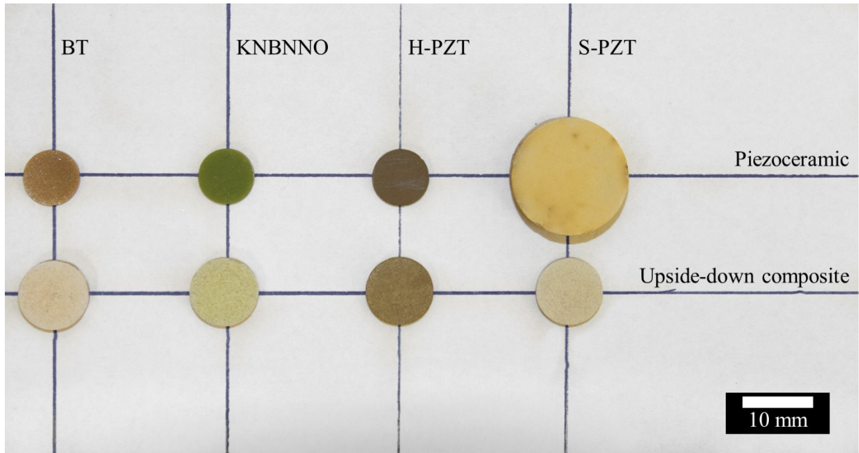
Figure S1. Pictures of sintered ceramic pellets and composite samples fabricated in this work.
