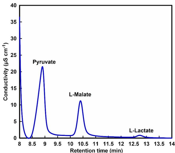
**Figure S4.** A chart of an ion chromatogram for L-malate concentration in the solution of sodium pyruvate (2.0 mM), manganese chloride (5.0 mM), NADH (2.0 mM), sodium bicarbonate (50 mM) and ME (0.7 U) in 5.0 mL of 500 mM HEPES buffer (pH 7.2).
