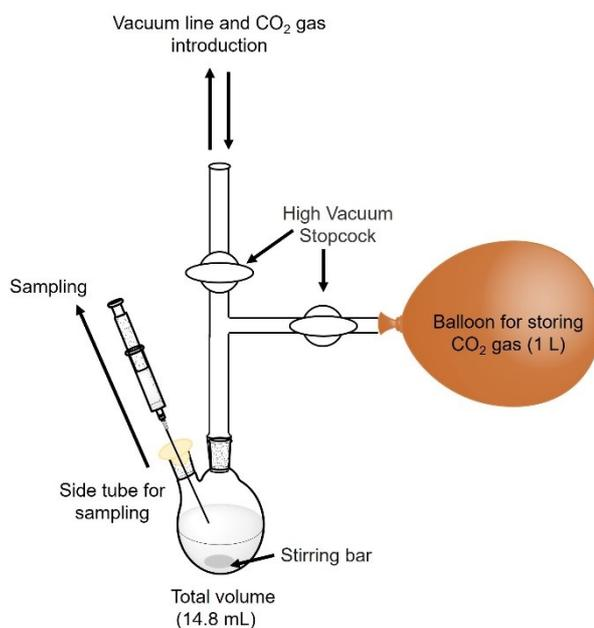
**Figure S1.** The experimental setup of the isobaric system for direct captured CO<sub>2</sub> gas and utilization to the reaction.
