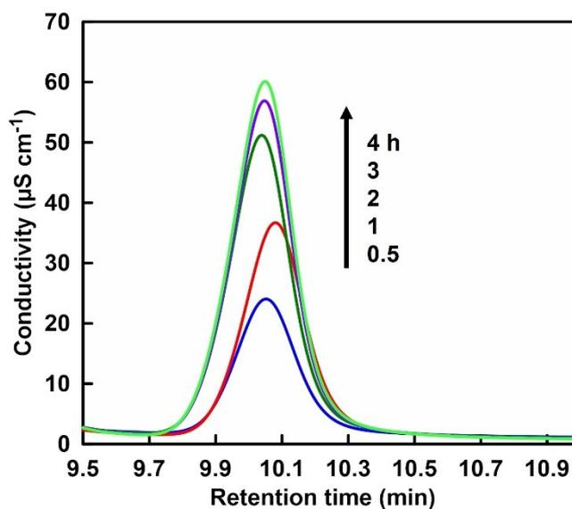
**Figure S3.** A chart of an ion chromatogram for L-malate concentration in the solution of sodium pyruvate (5.0 mM), manganese chloride (5.0 mM), ATP (5.0 mM), NADH (5.0 mM), acetyl-CoA (1.0 mM), PC (1.0 U) and MDH (10 U) in 5.0 mL of 500 mM HEPES buffer (pH 7.2). The gas phase: CO<sub>2</sub>.
