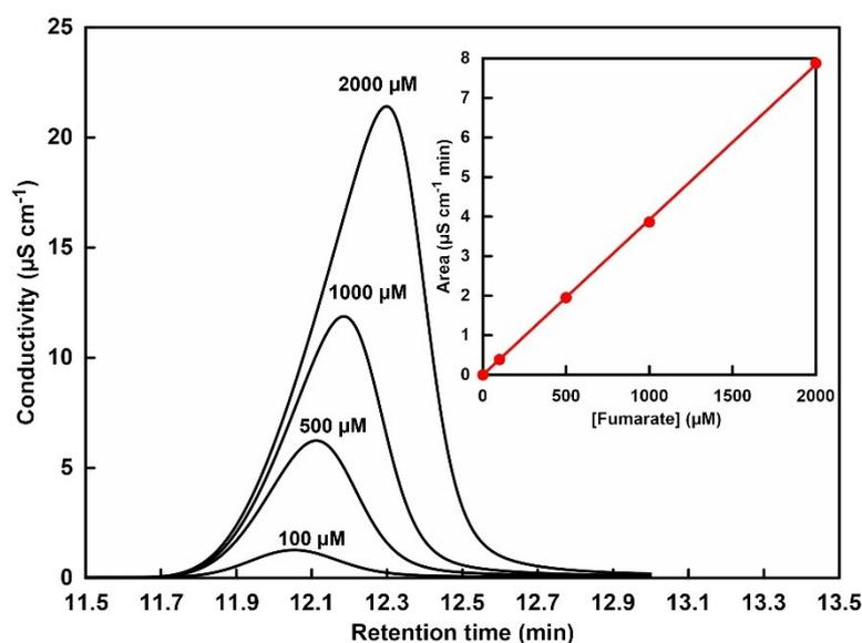
**Figure S5.** Chromatogram of sodium fumarate (0 – 2000  $\mu\text{M}$ ) in 50 mM-HEPES buffer (pH 7.0). Inset: Relationship between the fumarate concentration and the detection peak area.
