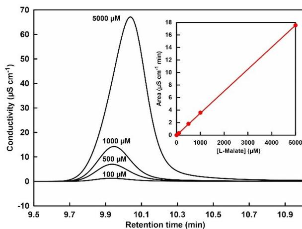
**Figure S2.** Chromatogram of sodium L-malate (0 - 5000  $\mu\text{M}$ ) in 50 mM-HEPES buffer (pH 7.0). Inset: Relationship between the L-malate concentration and the detection peak area.
