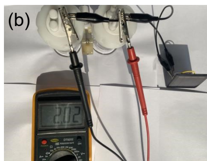
Fig. S24. Photographs of the overall water splitting device driven by a solar cell.
