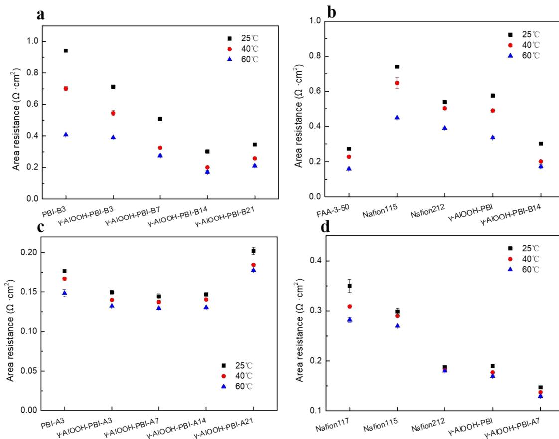
**Fig. S9.** Area resistance of  $\gamma$ -AIOOH-PBI composite membranes. a-b) Area resistance of different membranes at different temperatures in 1M KOH environment, c-d) Area resistance of different membranes at different temperatures in 3MH<sub>2</sub>SO<sub>4</sub> environment. Error bars are standard deviations obtained using three measurements from different samples.
