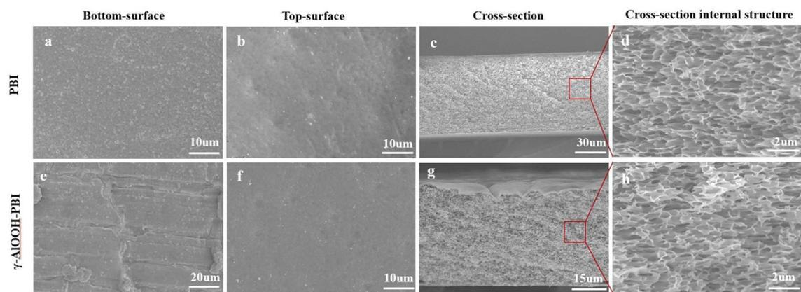
**Fig. S3.** SEM morphology of pristine PBI membranes and  $\gamma$ -AlOOH-PBI composite membranes.
