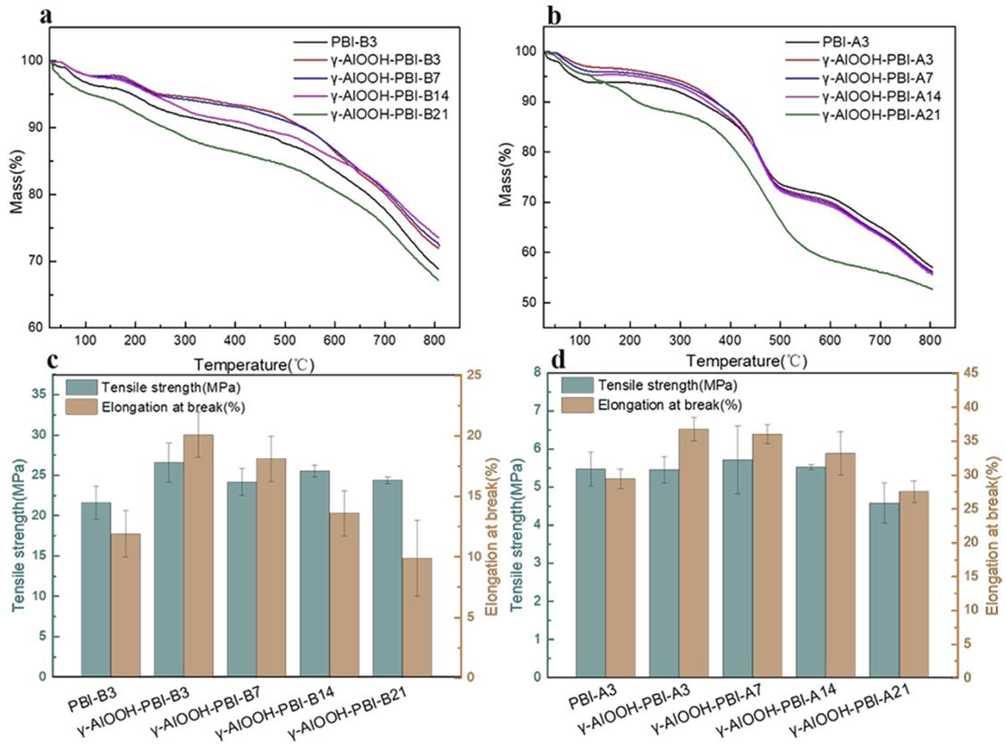
**Fig. S12.** a and b) TGA curves and c and d) stress-strain behaviors of pristine PBI and  $\gamma$ -AIOOH-PBI. Of note, B3, B7, B14, B21, A3, A7, A14, and A21 represent soaking days in alkaline and acid solution, respectively.
