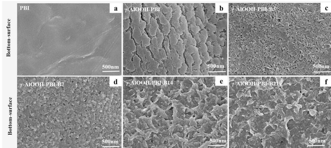
**Fig. S5.** SEM morphologies of pristine PBI and  $\gamma$ -AlOOH-PBI composite membranes. **a)** bottom-surface and bottom-surface of **a)** pristine PBI, **b-f)**  $\gamma$ -AlOOH-PBI composite membranes at different days of alkali immersion.
