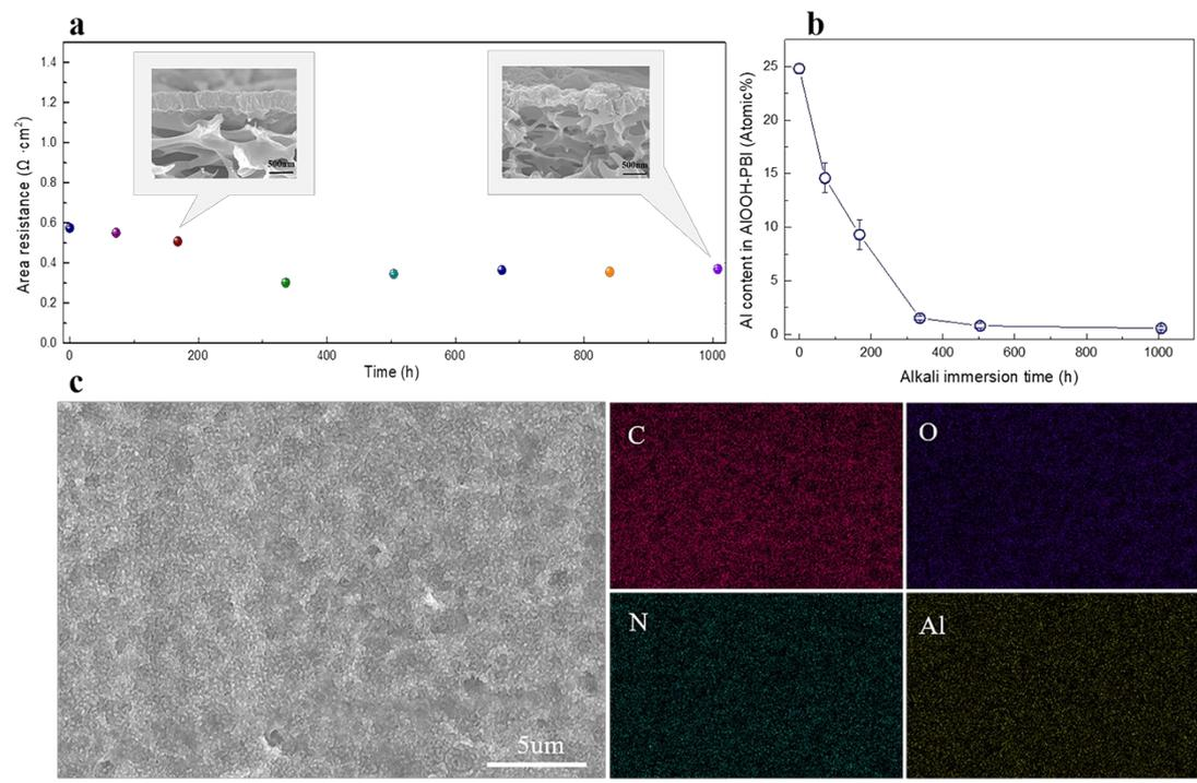
Fig.S7 **a**) The stability of  $\gamma$ -AlOOH-PBI composite membrane in 1MKOH environment; **b**) Variation curves of alkali immersion time and Al content in  $\gamma$ -AlOOH-PBI; **c**) The SEM image and elemental mapping of  $\gamma$ -AlOOH-PBI composite membrane after immersion in  $3\text{MH}_2\text{SO}_4$  environment at  $80^\circ\text{C}$  for 20h.
