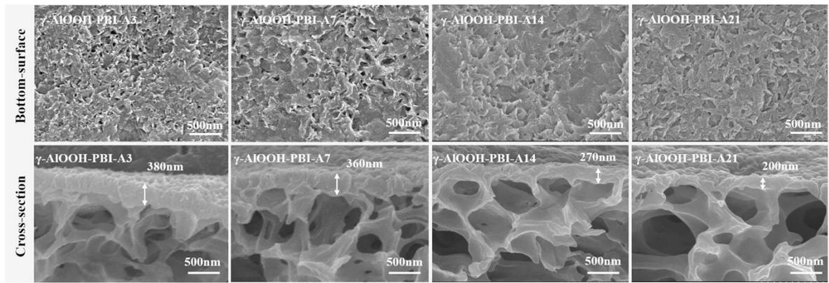
**Fig. S8.** SEM morphology of pristine PBI membranes and  $\gamma$ -AlOOH PBI composite membranes with different days of Acid immersion. A3, A7, A14, A21 are soaking days in in acid solution, respectively.
