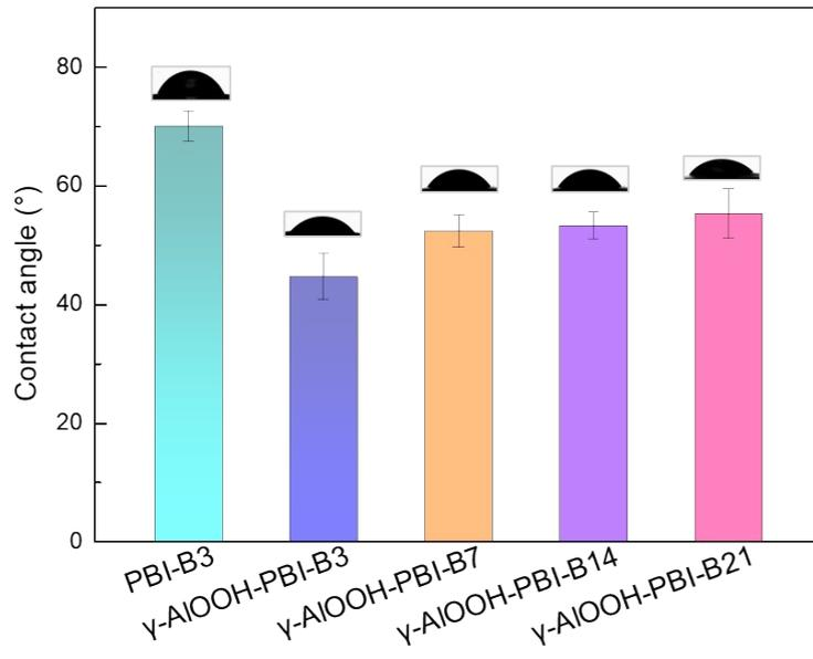
**Fig. S10.** The water contact angle of PBI-B3,  $\gamma$ -AlOOH-B3,  $\gamma$ -AlOOH-B7,  $\gamma$ -AlOOH-B14,  $\gamma$ -AlOOH-B21 membranes under dry state.
