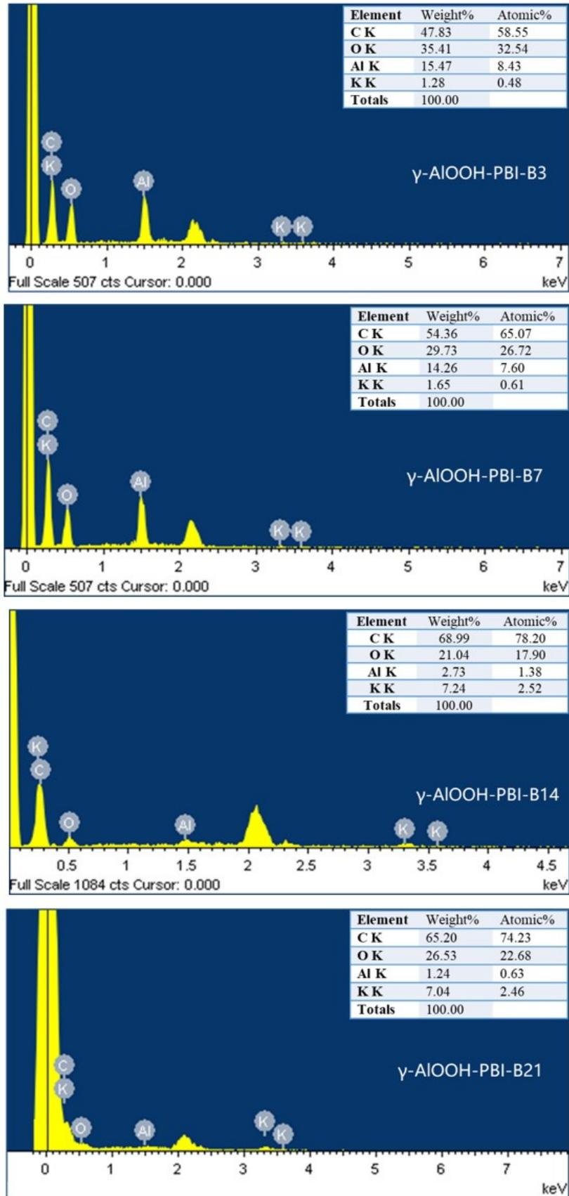
**Fig. S6.** EDS of  $\gamma$ -AIOOH PBI composite membranes with different days of alkali immersion. B3, B7, B14, B21 are soaking days, respectively.
