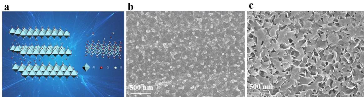
**Fig. S2.** SEM morphologies of aluminum-based surface nanostructures at different water bath temperatures. a) Schematic structure of  $\gamma$ -Al(OH)<sub>3</sub>, b)  $\gamma$ -Al(OH)<sub>3</sub>-50°C(SEM), c)  $\gamma$ -Al(OH)<sub>3</sub>-70°C(SEM).
