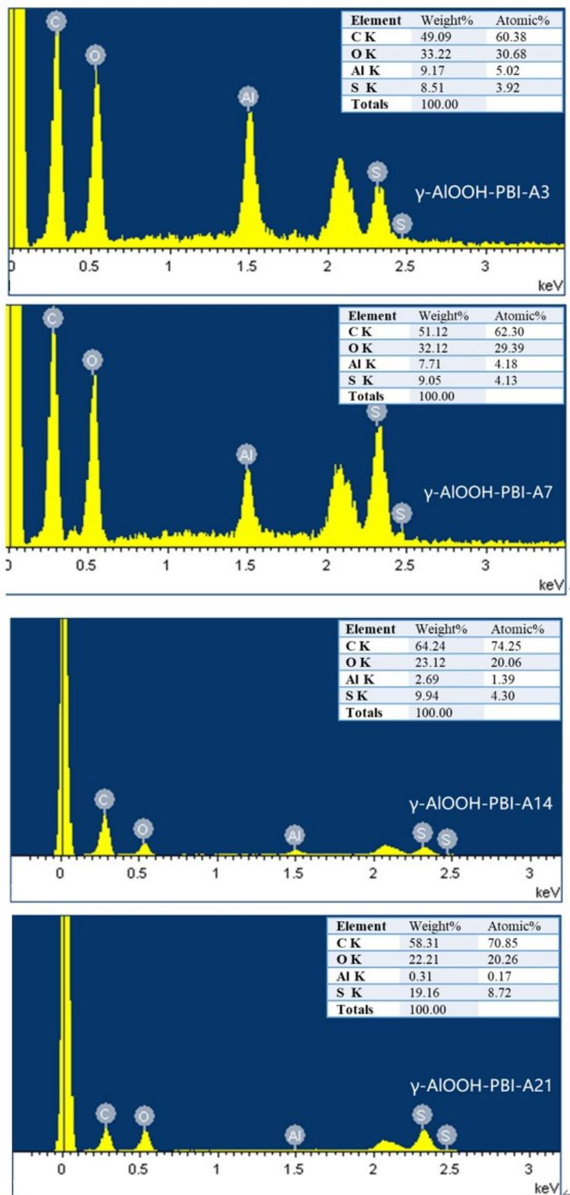
**Fig. S11.** EDS of pristine PBI membranes and  $\gamma$ -AlOOH PBI composite membranes with different days of acid immersion. A3, A7, A14, A21 are soaking days, respectively.
