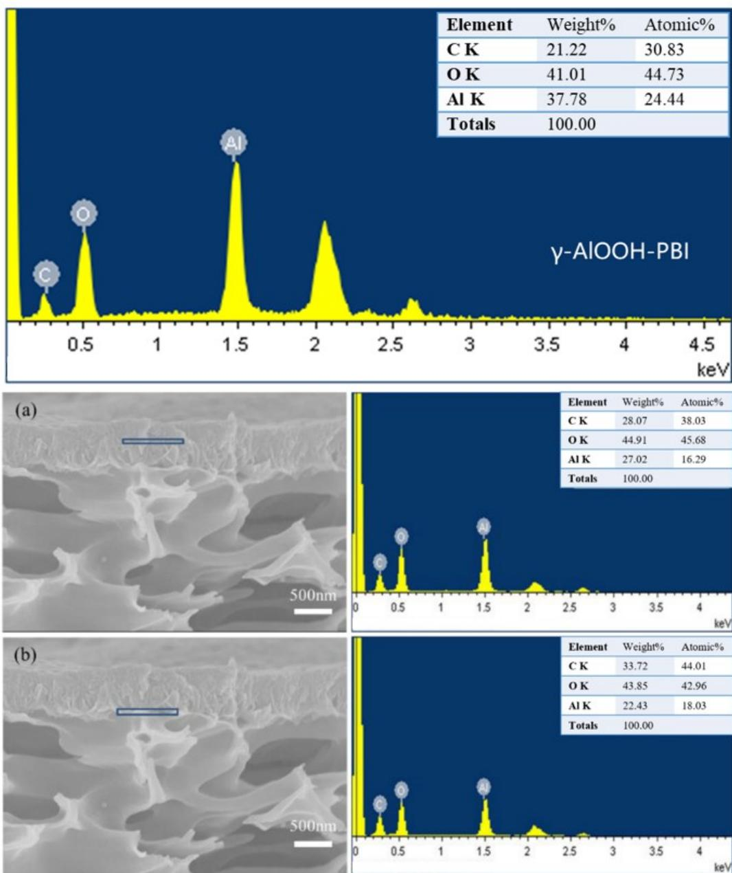
**Fig. S4.** EDS of  $\gamma$ -AlOOH PBI composite membranes and  $\gamma$ -AlOOH nanosheets a)  $\gamma$ -AlOOH nanosheet layers structure in the middle; b)  $\gamma$ -AlOOH nanosheet layers structure at the interface with the membrane.
