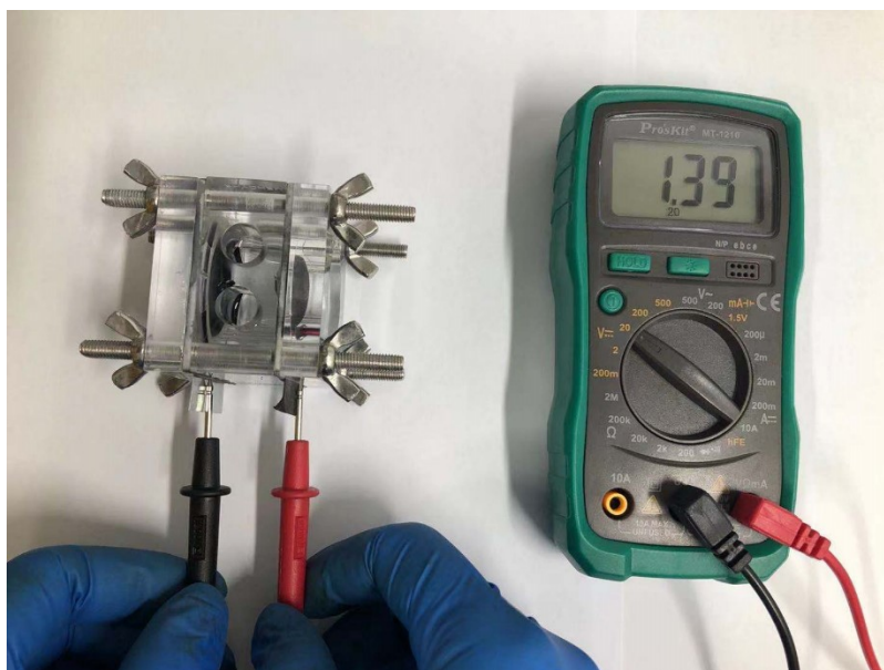
Fig. S26 Photograph of the 20% Pt/C-based Zn-air battery with an open circuit voltage of 1.39 V.
