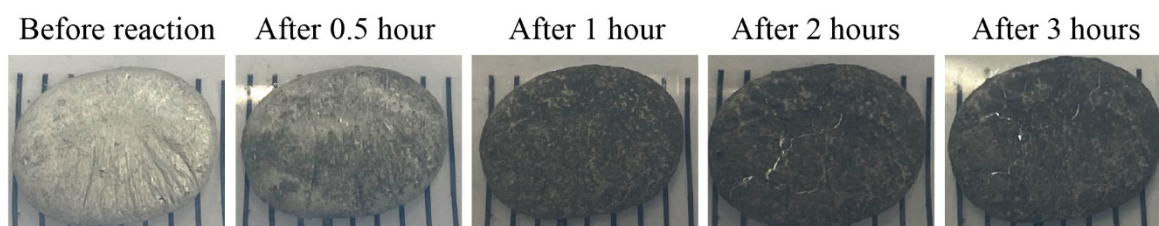
Fig. S1 Surface change with time of 0.2 wt. % Li-Ga alloy reacting with CO 2 in a syringe reactor.
