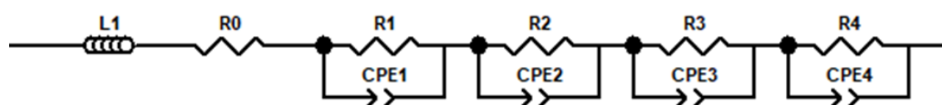
Figure S7. The equivalent circuit model proposed with the fitting on impedance spectra of p\text{H}_2\text{O} and p\text{O}_2 variations in oxygen electrode.
