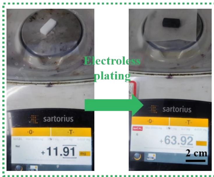
Fig. S2 Digital photos of Ni (left) and Ni@MF (right) on the Precision Balance.
