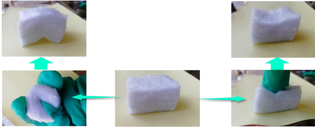
Figure S7 Photographs of the performance of QFF under bending and compression.
