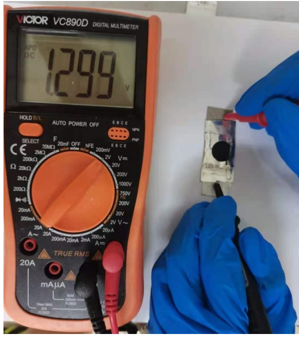
Fig. S17 Flexible soft-pack ZABs of open-circuit voltage.
