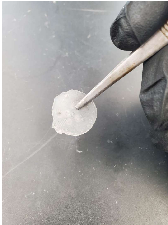
Figure S2. Optical picture of the polymer HNBR 35% ACN doped with 20 wt% PC.
