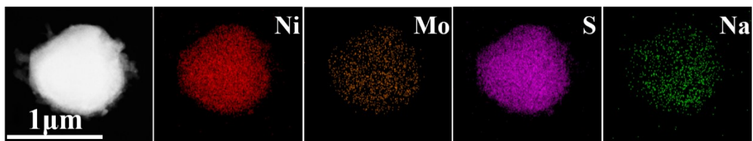
Fig. S16. EDS-mapping images of the \text{MoS}_2/\text{Ni}_3\text{S}_2@\text{C} electrode heterostructure electrode for SIBs at the full de-sodiation state.
