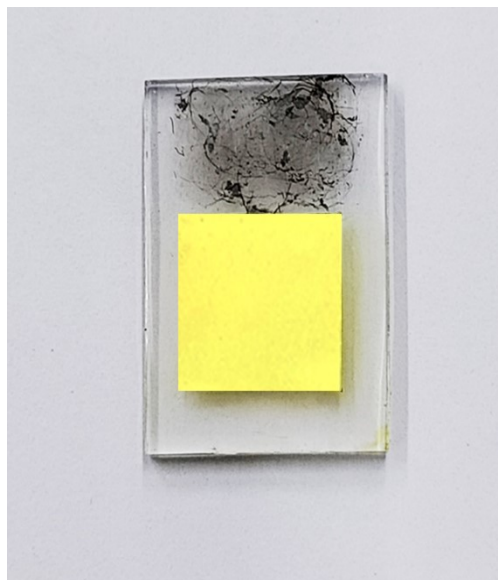
Figure S2: 1 cm 2 BiVO 4 /TiO 2 (BVT) photoanode with Pd nanoparticle as cathode (BVT-AL) wireless photocatalytic device. Just for the clarity of the Pd-particles in the photograph, deliberately large amount of Pd is coated; In the normal device, about ~10% is coated, compared to what is seen.
