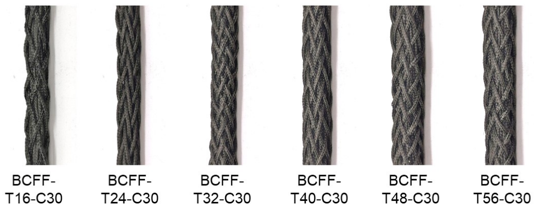
Fig. S9. The Optical images of the morphology of BCFF-Ts.
