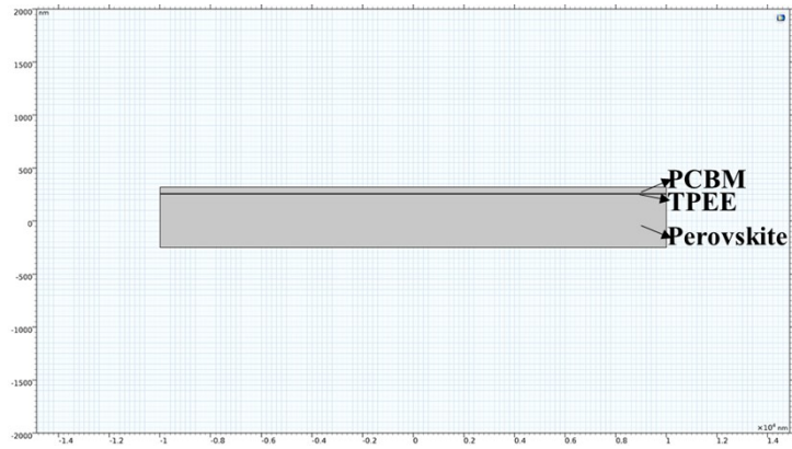
Fig. S7. The geometric model for bending simulation in finite element analysis. The design of this two-dimensional model is proportional, and the size of the geometric unit is 250 nm, which can match the grain size of perovskite films.
