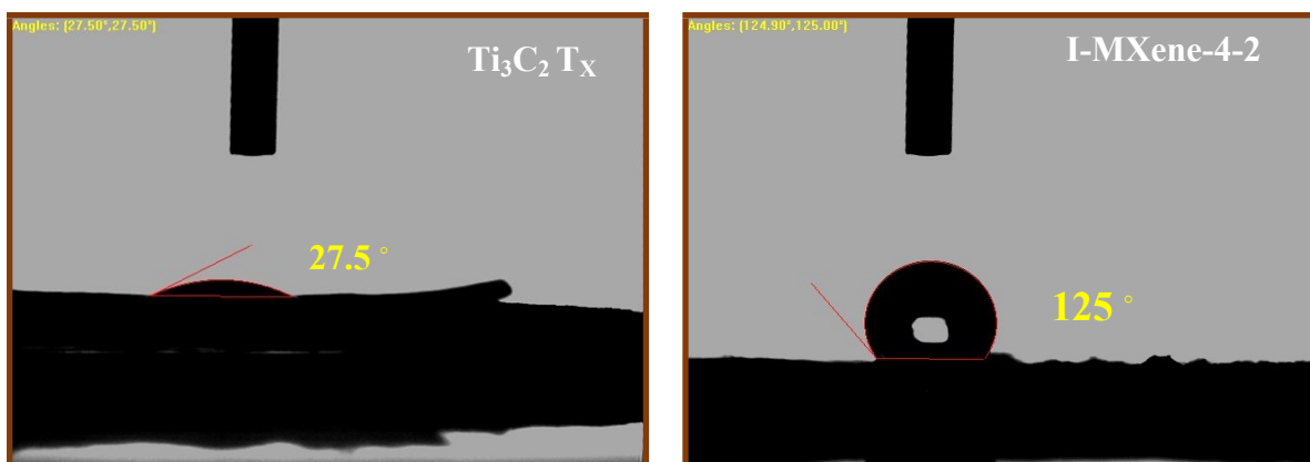
Figure S3. Water contact angle measurements on films of \text{Ti}_3\text{C}_2\text{T}_x MXene and I-MXene-4-2.
