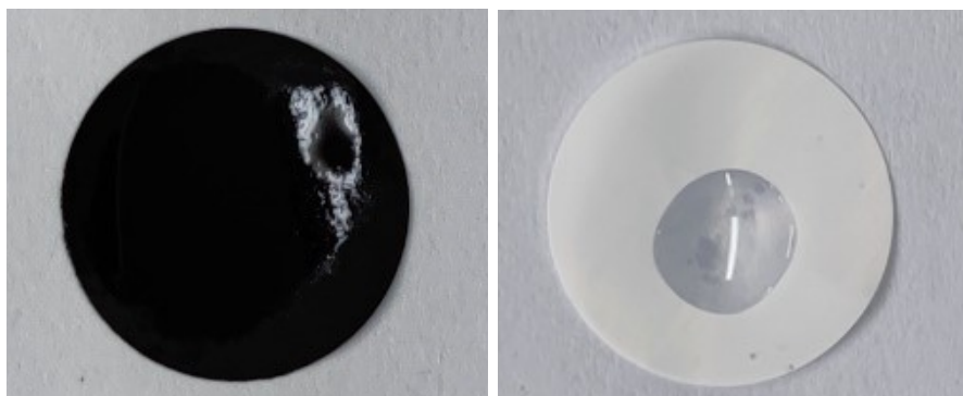
Fig. S11 The electrolyte wettability test of PP and c-Bi 2 Se 3 /a-BiO x -PP separators.
