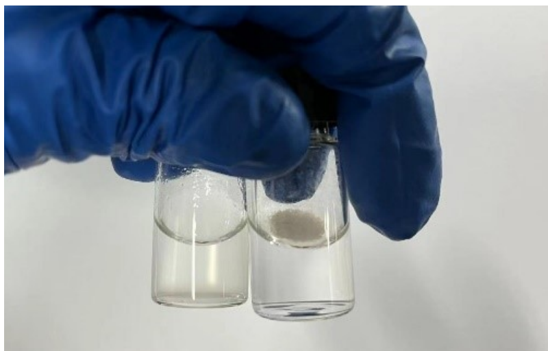
Fig. S1 Hydrophobic nano-SiO 2 was obtained by modifying hydrophilic nano-SiO 2 with octamethylcyclotetrasiloxane (D4).
