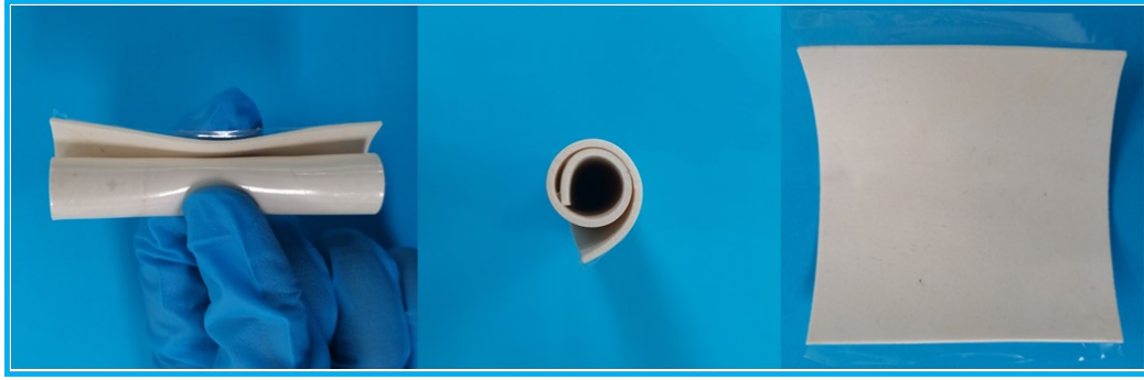
Fig. S8 Digital photos of NB20@M using as the phase change tape.
