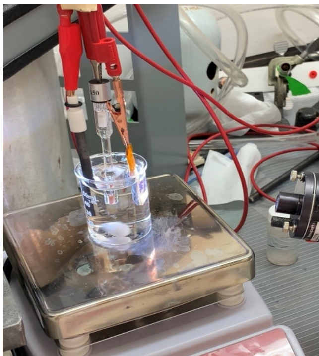
Figure S14 is the three-electrode set up of our PEC cell with simulated AM 1.5G illumination to the photocathode.
