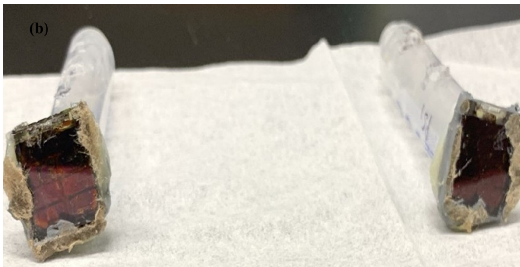
Figure S20 (a) showing the yellow color spots and discoloration seen in plain photocathode. (b) showing negligible discoloration after 120 hrs. continuous operation of PS based photocathode.
