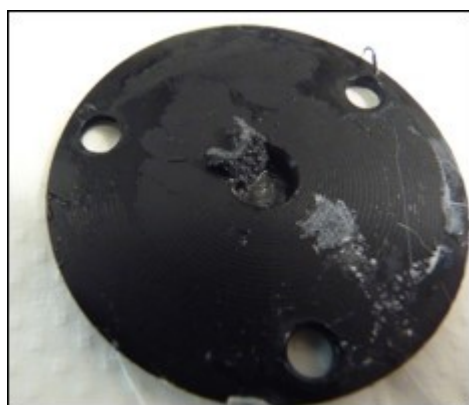
Supplementary Figure 28. Sludge formed on the anode while performing GCDC from a pristine additives-free electrolytes.
