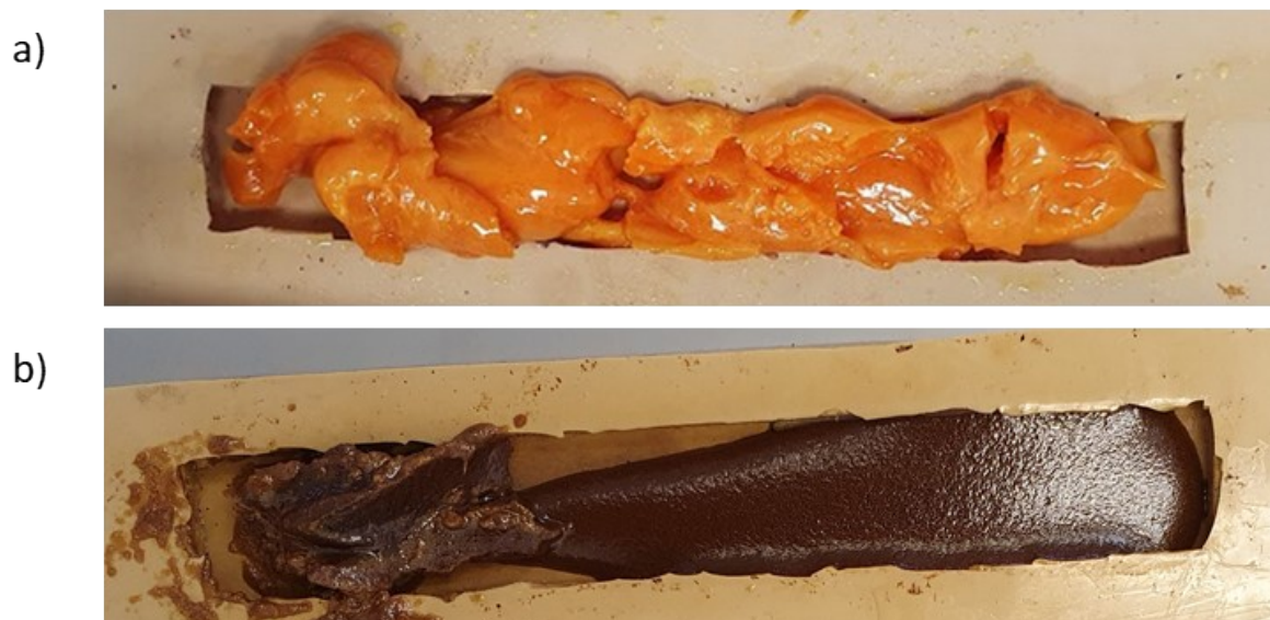
Fig. S3 Photos of S-DIB-cPBD pre-polymer a) when DIB is reacted before cPBD; b) when cPBD is reacted before DIB.
