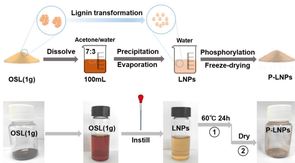
Fig. S2. The fabrication process of Phosphated Lignin Nanoparticles.
